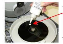
Place a small dab of compound at the 12 O'clock position for the second part of stage 1.
