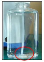
**IMPORTANT:**The Water Supply Tube should reach the bottom of the bottle.
