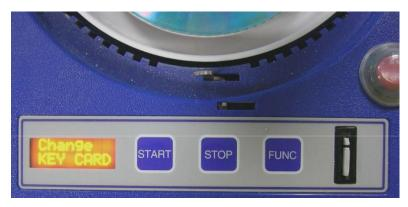
Turn OFF the Main Power Switch, exchange the KEY CARD (see page 9 for removal tips)
