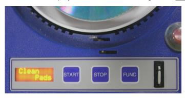
Exchange the pads for a clean dry pair and **press any button on the Operation Panel to clear the message**.
