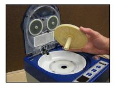
2. Take the polish tray out of the machine and wipe it with a damp cloth. You may also wash it in the sink, If needed.
