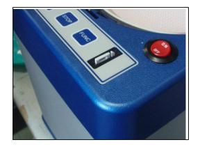
Be sure the KEY CARD is fully inserted into The KEY CARD slot by pushing it down and forward to lock it in place.
