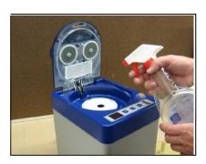
4. Wipeout the machine with a soft cloth to remove any polish build up.
