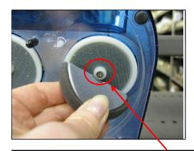
Bend the Pads lightly with fingertips, and fit the hole in the middle of the pad over the center pin of the Pad Holder
