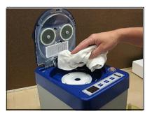
5. Spray the platen table assembly with glass cleaner and scrub with a toothbrush to clean it.
