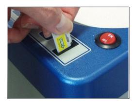
The KEY CARD should be inserted With arrow pointing down.
