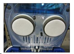
2. Press the center of the Pad lightly after placing it into the Pad Holder to attach the Velcro.
