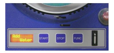
Add water to the Water Bottle, and then press any button on the Operation Panel to clear the alert indication.
